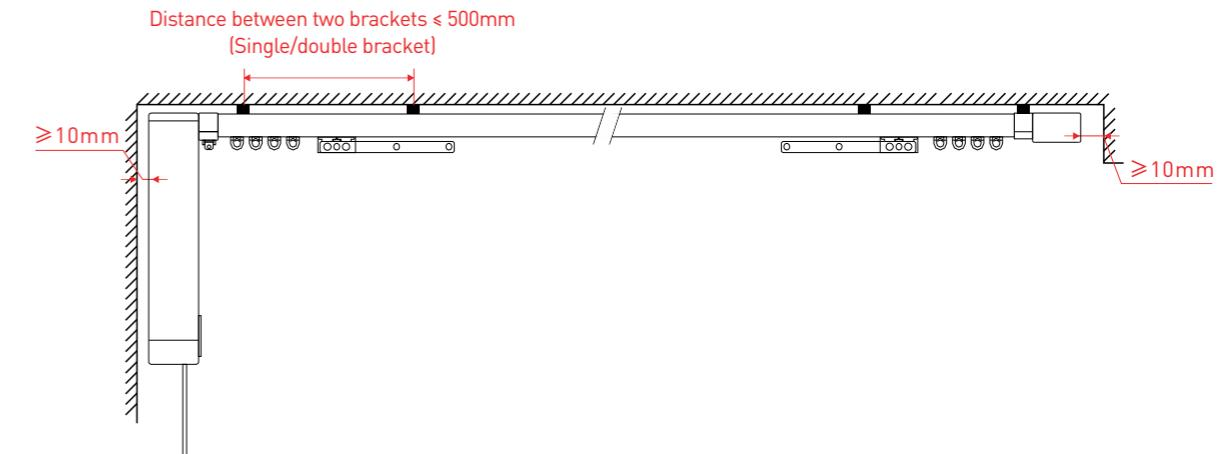
2. If you install a single curtain track, the prepared curtain box width should be no less than 100mm; If you install double curtain tracks, the prepared curtain box width should be no less than 180mm. The width can be adjusted according to the thickness and material of your curtain fabrics and your design.
