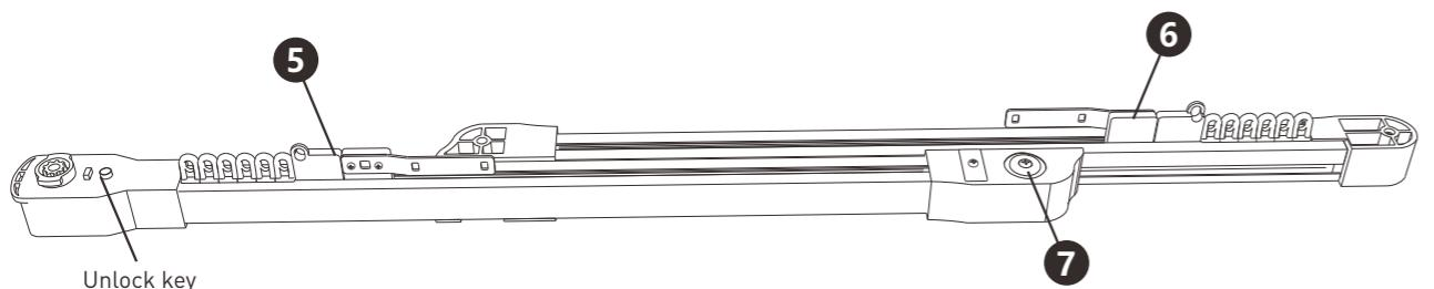
5. According to the track length you extend, install an appropriate number of brackets. Single bracket should be inserted around every 50 centimeters of a single track. Likewise, double bracket should be inserted around every 50 centimeters of the double tracks. After the brackets are inserted, the track pre-installation is completed.
