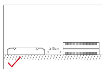
Please not place the products on LED drivers. The distance between the product and the driver should be  $\geq 15\text{cm}$  so as not to affect heat dissipation and shorten the lifespan of the products.
