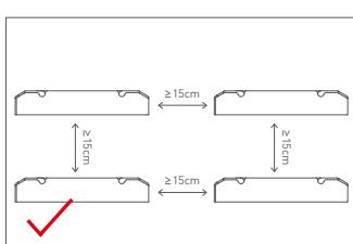
Please do not stack the products. The distance between two products should be  $\geq 15\text{cm}$  so as not to affect heat dissipation and the lifespan of the products.
